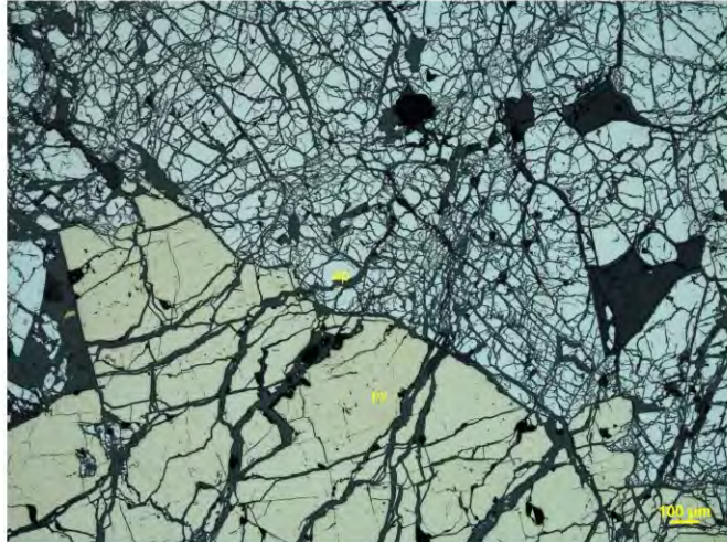
Photomicrograph 4a: Xenomorphic crystals of pyrite (py) are intergrown with arsenopyrite (ap). The arsenopyrite and the pyrite are strongly fractured. Plane-polarized reflected light.
