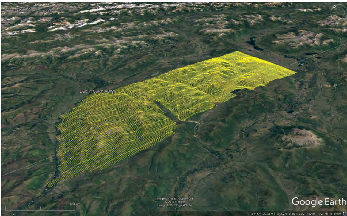
Figure 4: Terrain View – Dublin Gulch/VBW with actual flight lines displayed in yellow.
