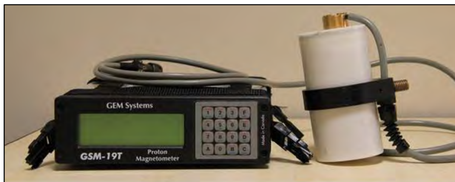
Figure 19: GEM GSM-19T proton precession magnetometer.
