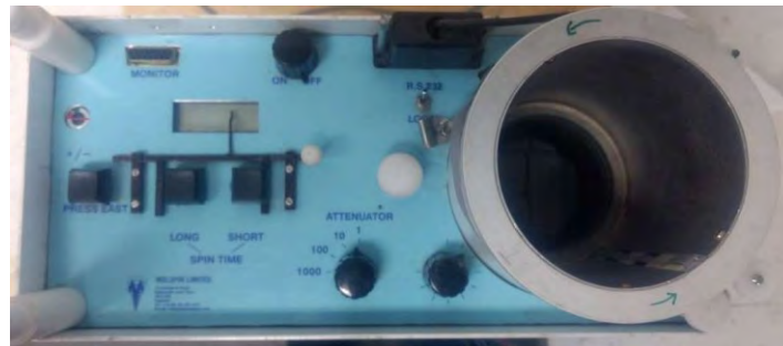
Figure 4: Mospin instrument used to measure remnant magnetism
