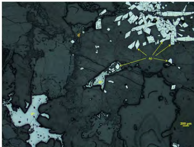
Photomicrograph 6b: Fine-grained crystals of arsenopyrite (ap) define irregular crystal clusters. The galena (gn) occurs as rare amoeboid crystals. Plane-polarized reflected light.
