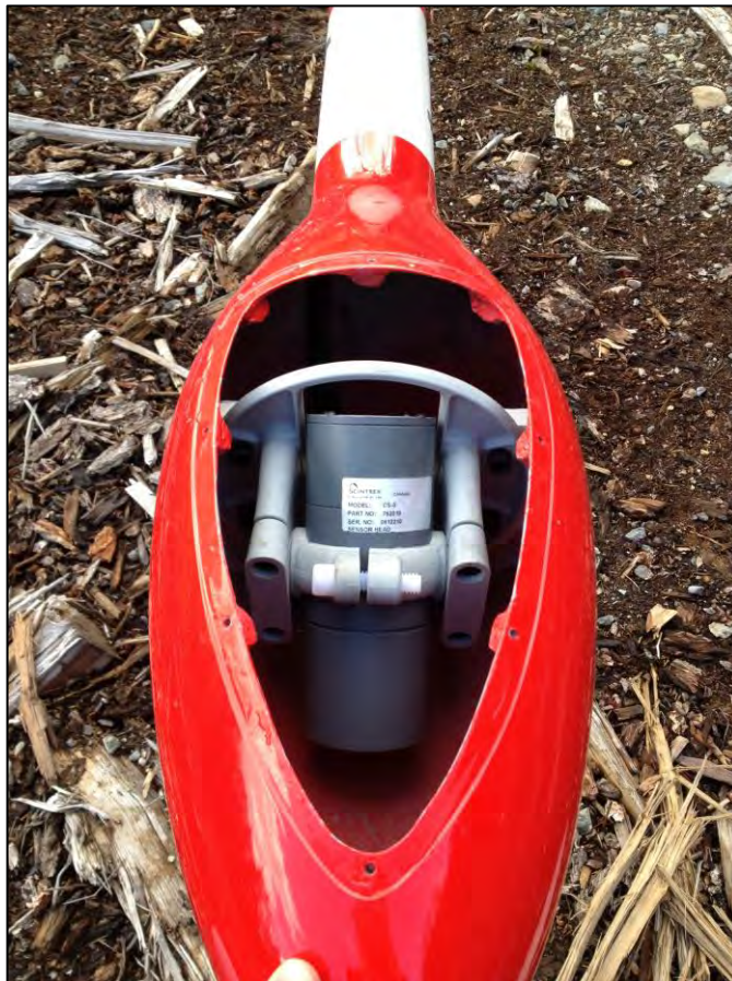
Figure 17: Scintrex cesium vapor CS-3 magnetometer mounted on the front of the helicopter in an approved “stinger” configuration. Sensor oriented 45° from vertical.
