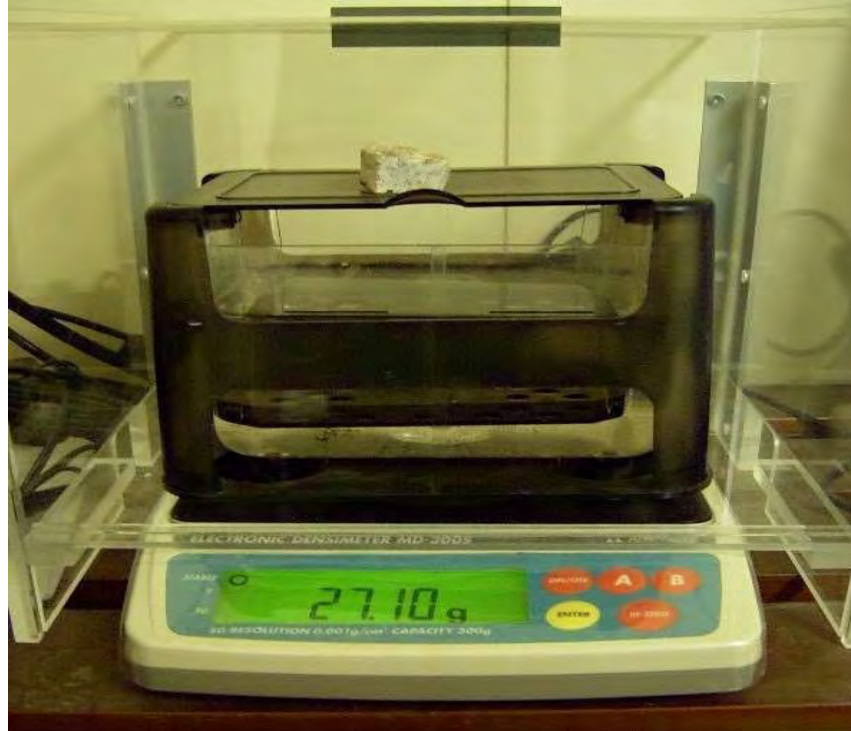
Figure 1: Electronic Densimeter MD-300S used for specific gravity readings
