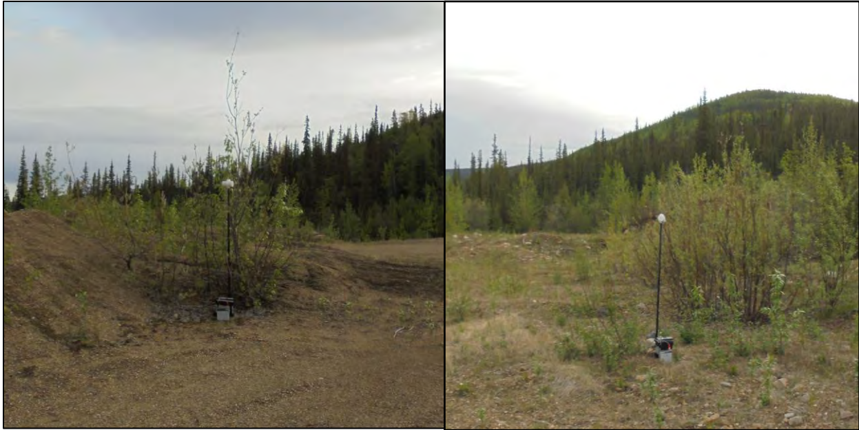
Figure 8: GEM 4 (left) and GEM 5 (right) magnetic base stations located in the field far away from metallic items/objects.
