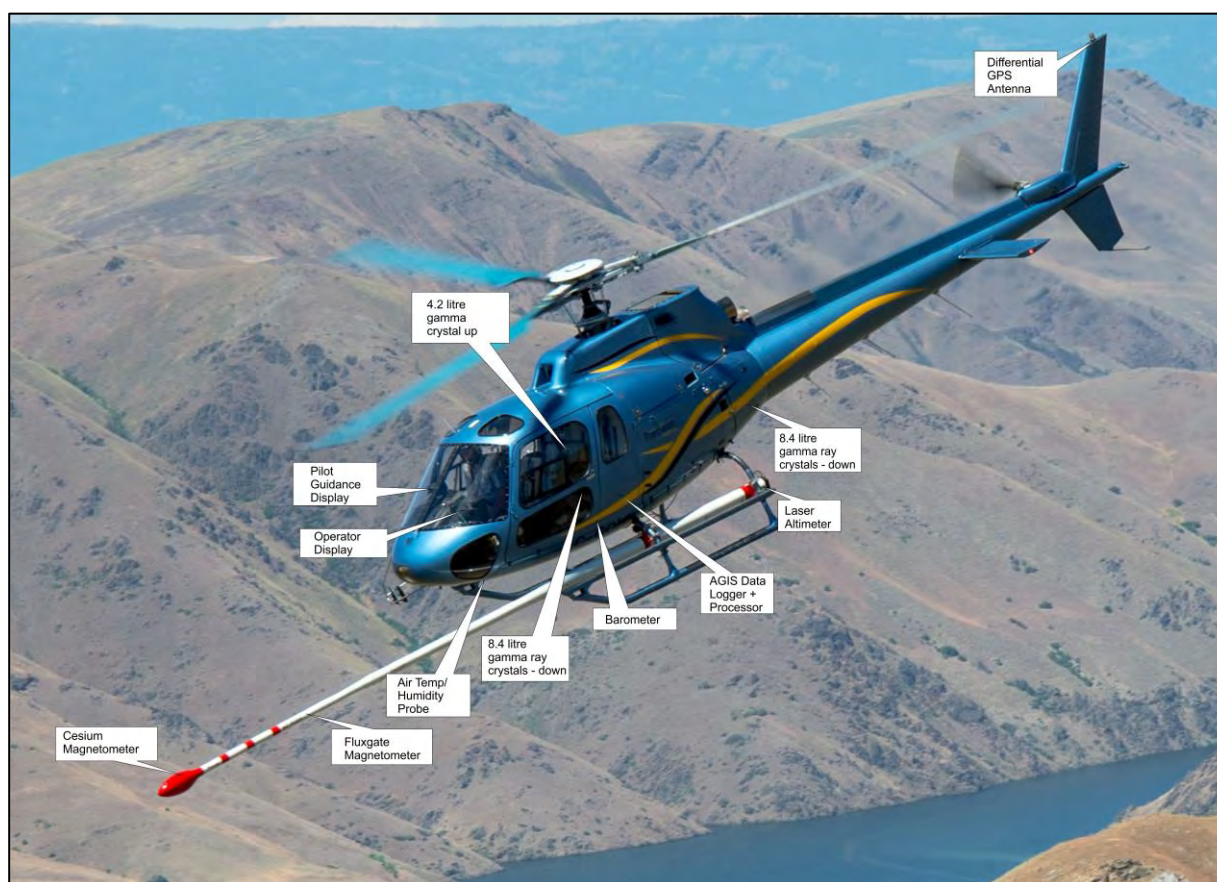
Figure 15: Geophysical survey helicopter equipped with geophysical equipment.
