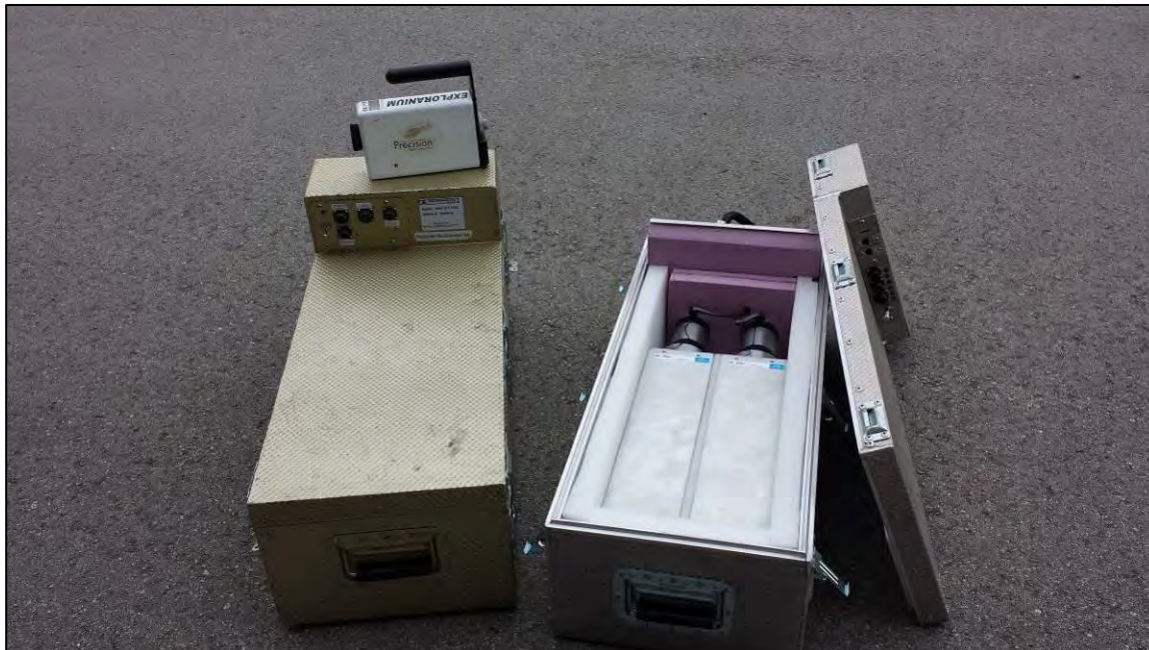
Figure 18: GRS-10 Thallium-activated Sodium Iodide gamma spectrometer crystal pack. The open unit on the right shows two individual 4.2 liter detectors.
