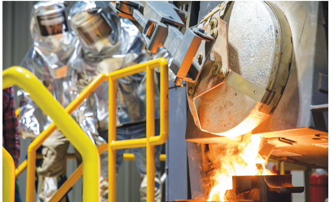
Pouring the molten gold heated to 1100 degrees C.
